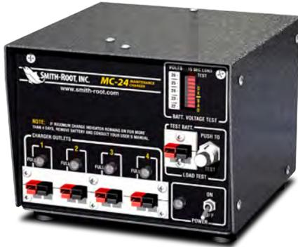
battery and identify low charged and worn-out batteries. Charging lead-batteries using the MC-24 takes between two and four days. It is also an excellent cost-effective alternative to purchasing multiple battery chargers because it can recharge four batteries at once (the MC-24 is NOT designed to maintain or charge lithium batteries).
